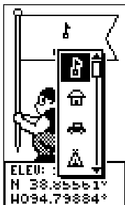
The Mark Waypoint Page allows you to change the symbol for the waypoint.
