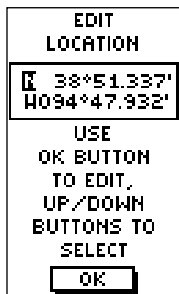
The EDIT LOCATION Page displays on-screen instructions explaining how to edit the waypoint location.
