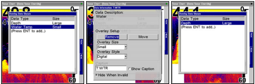
Overlay Data Shown with Water Temp selected (left). Remove button highlighted (center). Water Temp has been removed from Overlay Data Shown menu (right).
