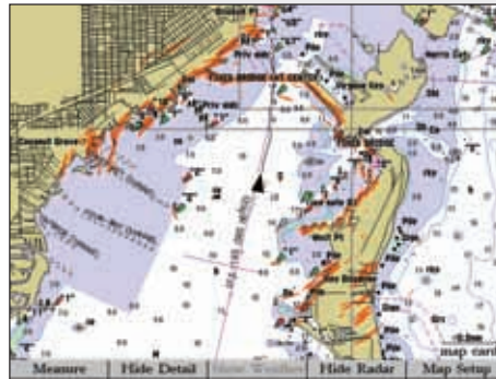
As an aid in locational awareness, the GMR 20/40 radar image can be overlaid on the moving map cartography display.
